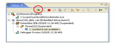
The application will start, run all of our ARM initialization code and stop at the start of **main()**. Note that in the Debug view, the **Thread[0]** is suspended at line 46 of main. With embedded cross development, we only have one execution thread. Code targeted for the PC platform can have multiple threads of execution.
