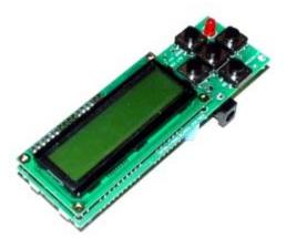
This is the Olimex LPT-MT development board; it has everything the prototype board above includes plus a LCD display and four pushbuttons to experiment with. It costs about \$79.95 plus \$2.95 for the wall-wart power supply.
