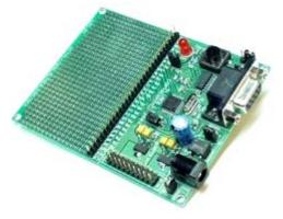
This is the Olimex LPC-P2106 prototype board. Everything is done for you. There's a power connector for a wall-wart power supply, a DB-9 serial connector and a JTAG port. It costs about \$59.95 plus \$2.95 for the wall-wart power supply.
