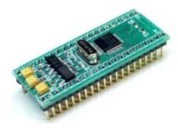
This is the Olimex LPC-H2106 header board. You can literally solder this tiny board onto Radio Shack perfboard, attach a power supply and serial cable and start programming. It costs about \$49.95 Obviously, it requires some soldering to get started.
